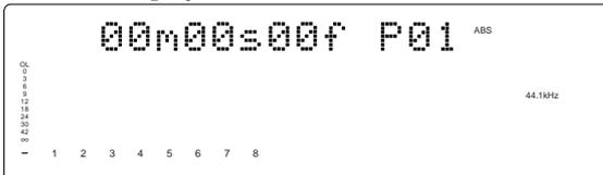
At this time if you press the DISP SEL key, the Disk Remain display will appear. (Both recordable time and hard disk capacity remaining will be converted to mono track and expressed in time and megabytes.)
