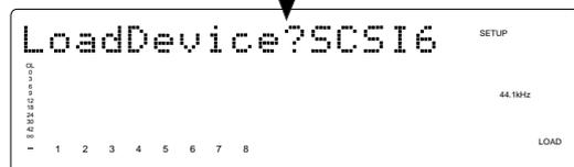
**4. Rotate the JOG dial to select a flashing “SCSI 6.”**
