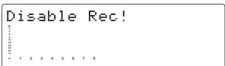
**Action to take:** Change the "Off" (recording) "Rec Protect ?" setting in Setup mode.
