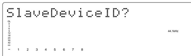
\* Press the select key of the RECORD TRACK according to the ID number of the slave machine.
