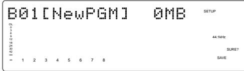
Pressing the EXECUTE/YES key will start save operations and then the following indication will appear. This indicates that the song data of the current drive selected is being saved on the B01 backup disk. The disk space necessary to save the data is counted down while the data is being saved.
