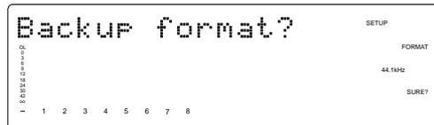
If it is okay to proceed formatting, then execute the formatting process as done in the above case. If it is not okay to proceed formatting, then turn the JOG dial to select [Eject] to eject the disk.
