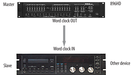
Figure 4-21: Slaving another digital audio device to the 896HD via word clock. For the 896HD clock source, choose any source besides word clock, as it is not advisable to chain word clock.
